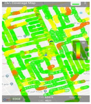
Fig(7) Drive test and walk test to collect data from 2G cell
