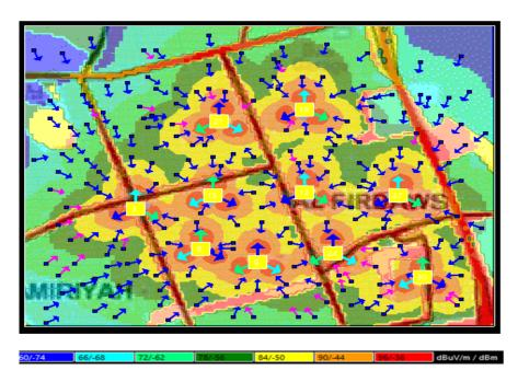
10 towers are deployed in real locations 2G and each tower contains 3 sectors, as well as more than 200 test points, are published by ICS Telecom program, as shown in figure (3):
