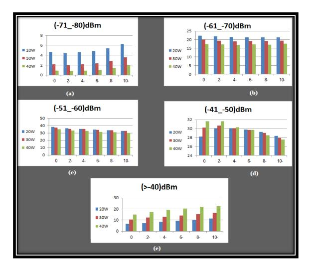
Fig(15) (a, b, c, d, and e) : Percentage of Coverage for each range within a different power and tilt
