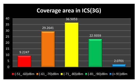
Fig(6) Simulation of coverage area for 3G network (power=20w, Tilt=-10)
