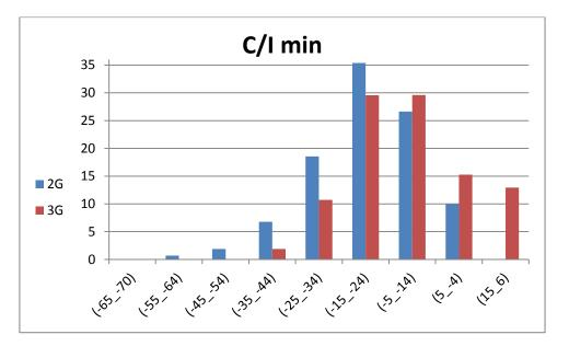
Fig(14) Comparison C/I between 2G and 3G cells
