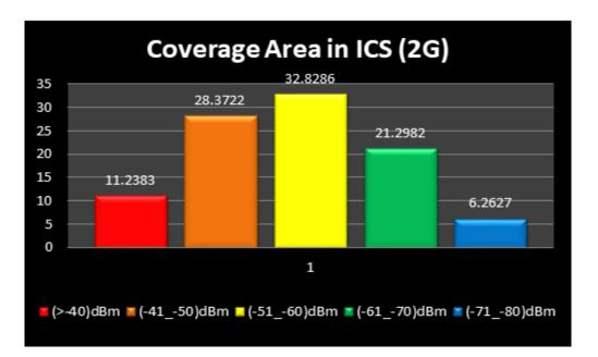
.Fig(5) Simulation of coverage area for 2G network (power=20w, Tilt=-10)
