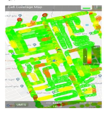
Fig(8) Drive test and walk test to collect data from 3G cell
